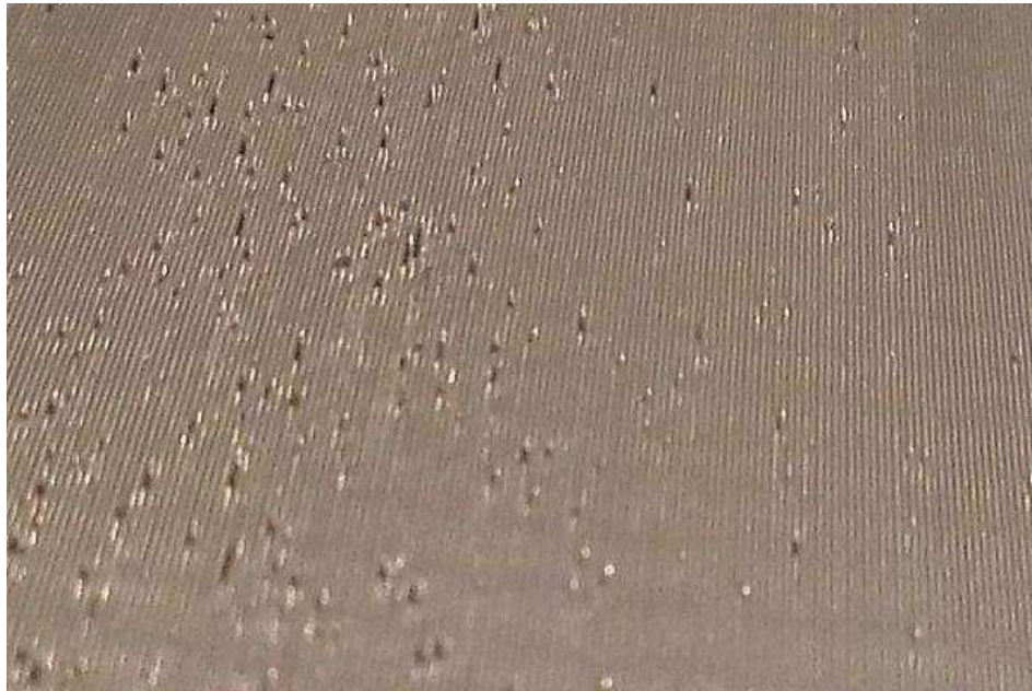
Voids in 3D Printed parts. Source: idig3dpriitning.com
