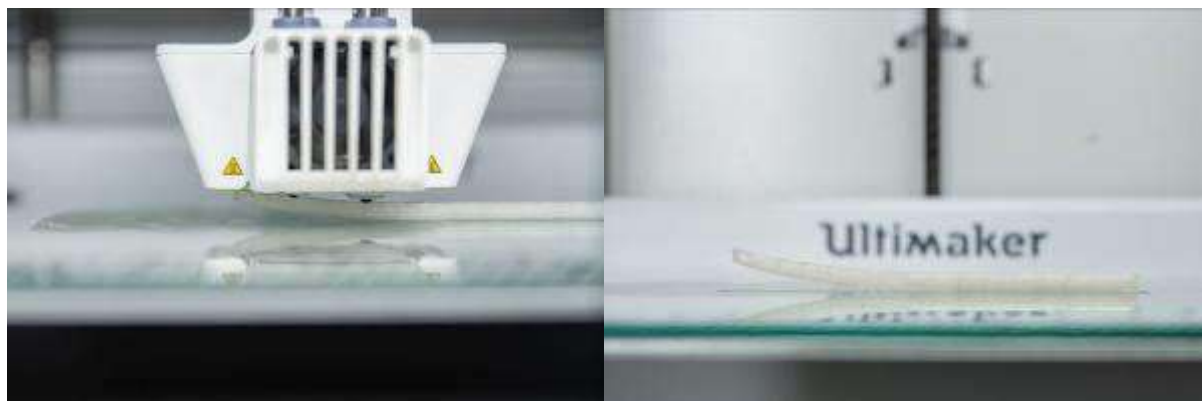
Figure 2: Nylon warping due to insufficient bed adhesion, one side is printed on regular glue stick, the other on Magigoo PA adhesive
