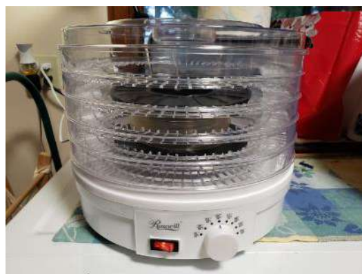
A food dehydrator turned into a filament dryer, Source : bluepapertech.com
