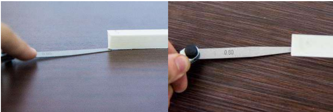
Figure 13: Measuring the warp on the edge of the wedge print using a feeler gauge
