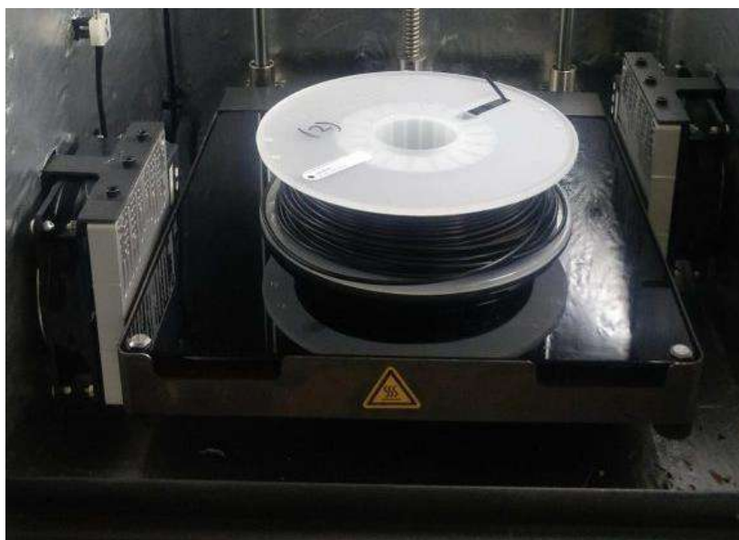
A filament being dried inside a heated 3D printer chamber.
