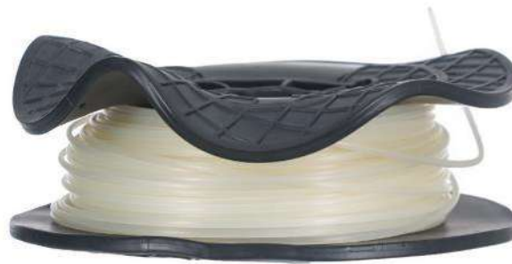
Warped filament spool due to excessive heating in an oven
