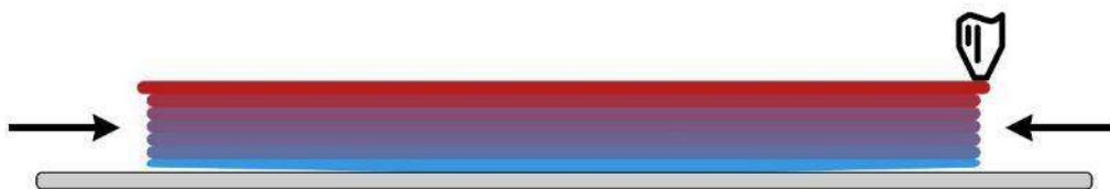
Figure 5: Print warp due to thermal gradient
