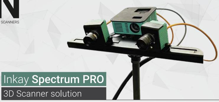
Inkay Spectrum PRO is a professional optical 3D scanner designed for scanning complex technical objects. It is ideal for reverse engineering, quality control, inspection and industrial design. High detalization and precision of 3D models are provided by high-resolution cameras, a LED projection module, structured blue light technology and unique data processing algorithms.
