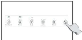
Press the power button. When starting the machine, the default mode is Auto. When the purifier is turned on, the Negative Ion function automatically turns on
