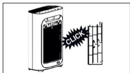
5. Reinstall the filter in the air purifier and reinstall the back part.
